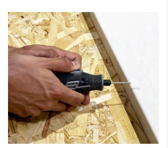
Using the rotary tool, carve the area making a uniform indentation. Clean the area with alcohol.
