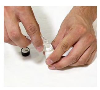
Pour Paint (A) & Texture (B) into Catalyst (C). Close Catalyst bottle (C) and shake for one minute to mix contents.
